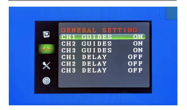
Using button 5 or button 7 to choose CH1/CH2/CH3's "GUIDES" settings, use button 1 or 3 to turn on and off it. After trigger wire is activated, the parking lines will be turned on or off.
