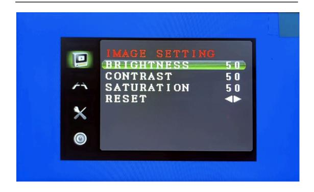
Using button 5 or button 7 to choose "BRIGHTNESS" or "CONTRAST" or "SATURATION" or "RESET" settings, use button 1 or button 3 to set the value. Use button 1 or button 3 to restore default settings;
