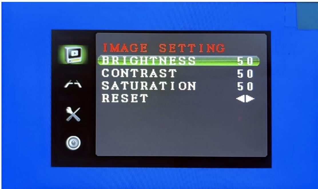
Using button 6 or button 7 to choose "BRIGHTNESS" or "CONTRAST" or "SATURATION" or "RESET" settings, use button 2 or button 4 to set the value. Use button 2 or button 4 to restore default settings;
