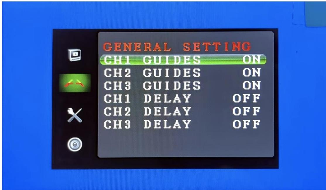
Using button 6 or button 7 to choose CH1/CH2/CH3's "GUIDES" settings, use button 2 or 4 to turn on and off it. After trigger wire is activated, the parking lines will be turned on or off.
