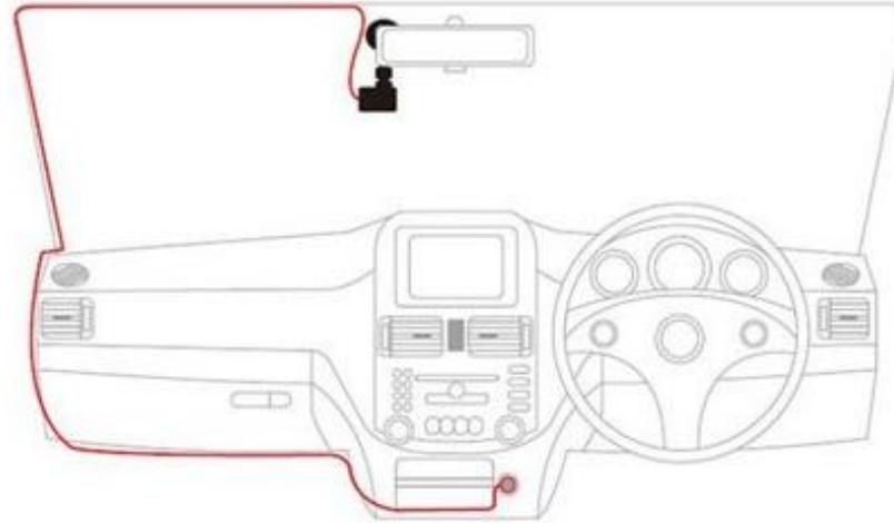
Note: The wiring of the car charger can be hidden by installing according to the picture above.
